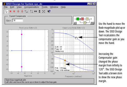
Figure 4-7: Root Locus and Bode Plots for the DC Motor
