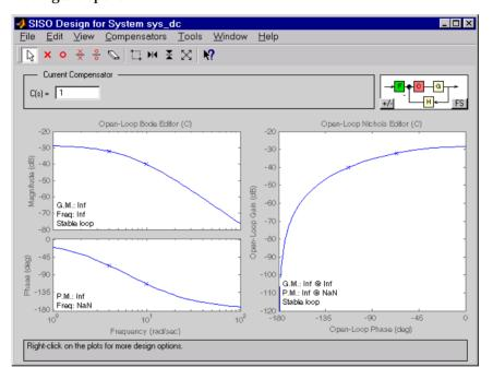
Figure 4-42: SISO Design Tool with a Nichols Plot
