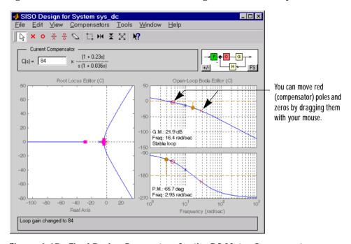
Figure 4-15: Final Design Parameters for the DC Motor Compensator
