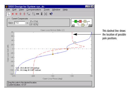
Figure 4-47: Moving the Lead Network's Pole
