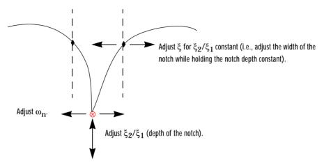
Figure 4-20: A Close Look at Notch Filter Parameters
