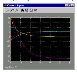
Figure 4-60: The Control Inputs for the LQG Tracking Problem
