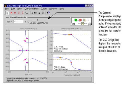
Figure 4-32: The Result of Adding a Complex Pair of Poles to the Compensator
