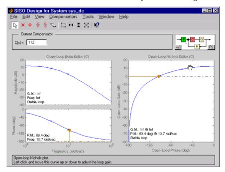
Figure 4-43: Adjusting the Compensator Gain by Moving the Nichols Curve
