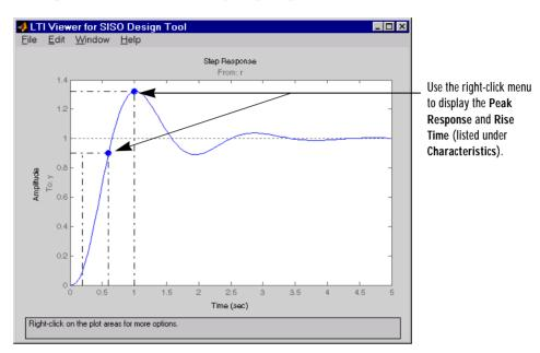
This figure shows the closed-loop step response.
