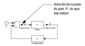
Based on the location of the Input Point and Output Point blocks, you might think that the analysis model specified by these blocks is simply the plant model, P. However, due to the feedback loop, this analysis model is actually the closed-loop transfer function P/(1+PK).
