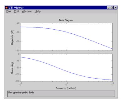
Figure 3-8: Bode Plot for the DC Motor Model
