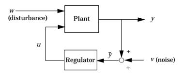
The goal is to regulate the output y around zero. The plant is subject to disturbances w and is driven by controls u. The regulator relies on the noisy measurements  $\bar{y} = y + v$  to generate these controls. The plant state and measurement equations are of the form
