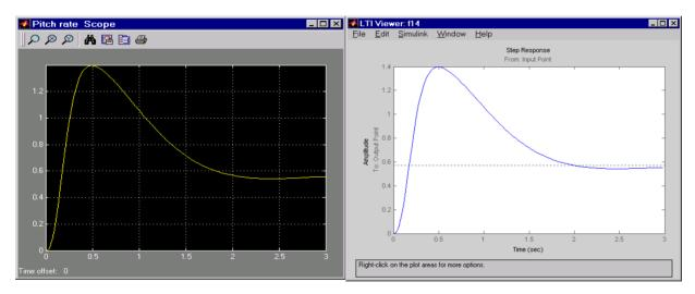
Figure 3-23: Comparison of Step Responses from Stick Input to Pitch Rate for the Nonlinear and Linear F14 Models, Respectively
