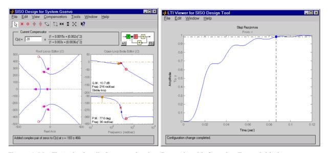
Figure 4-33: Electrohydraulic Servomechanism Example with Complex Zeros Added
