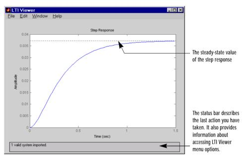
The picture below shows the LTI Viewer with a step response for the DC motor example.
