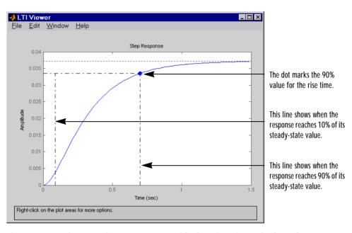
The LTI Viewer calculates and displays the rise time for the step response.
