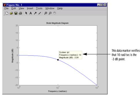
This figure shows the Bode magnitude of the shaping filter.
