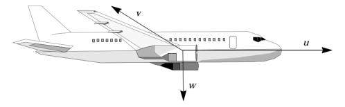
Figure 4-55: A Body Coordinate Frame for an Aircraft
