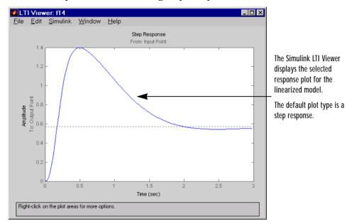
Figure 3-22: Step Response from Stick Input to Pitch Rate for the Linearized F14 Model
