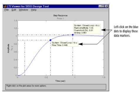
**Characteristics** and then **Rise Time** and **Peak Overshoot**. This figure shows the plot with the rise time and overshoot denoted by large dots on the curve.
