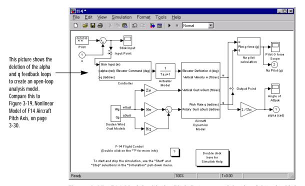
Figure 3-25: F14 Model with the Pitch Rate, q, and Angle of Attack, Alpha, Feedback Paths Removed
