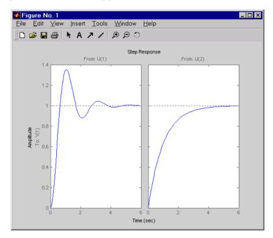
Figure 3-13: Step Responses for a MIMO Model
