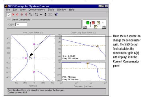
Figure 4-29: Changing the Compensator Gain in the Root Locus Plot
