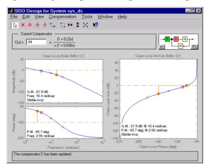
Figure 4-48: Final Nichols Plot Design for the DC Motor Compensator
