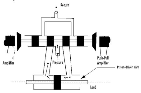
Figure 4-24: An Electrohydraulic Servomechanism
