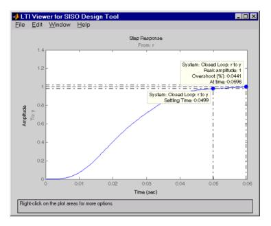
Figure 4-36: Closed-Loop Step Response for the Final Design of the Electrohydraulic Servomechanism Example
