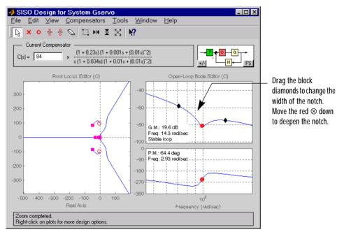
This figure zooms in on the notch filter to show the adjustable parameters.
