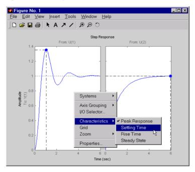
Figure 3-14: Using the Right-Click Menu in a Step Response Plot
