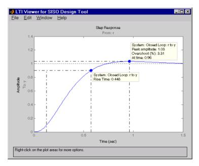
Figure 4-49: Closed-loop Step Response for the Final Compensator Design
