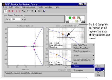
Figure 4-12: Zooming in on the X-Axis of the Bode Plots
