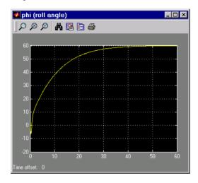
Figure 4-58: Tracking the Roll Step Command
