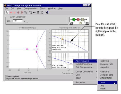
Figure 4-13: Adding a Lead Network to the DC Motor Compensator Using Right-Click Menus
