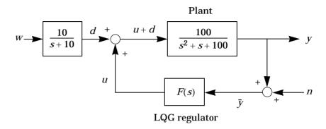
Figure 4-51: Simple Regulation Loop
