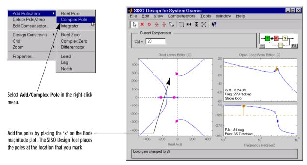
Figure 4-31: Adding a Complex Pair of Poles to the Compensator
