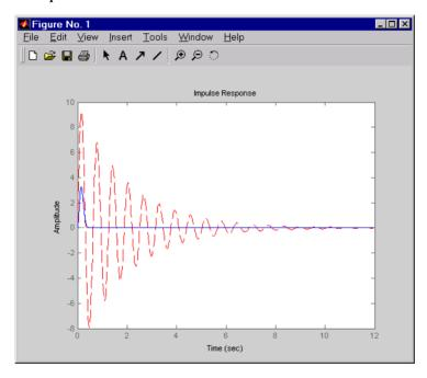
Figure 4-53: Comparison of Open- and Closed-Loop Impulse Response for the LQG Example
