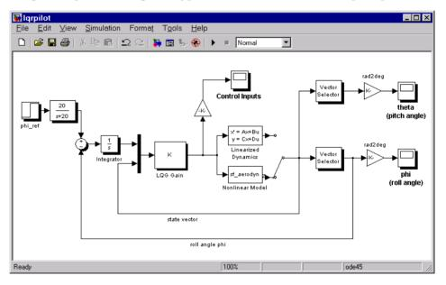
Figure 4-54: A Tracking Loop
