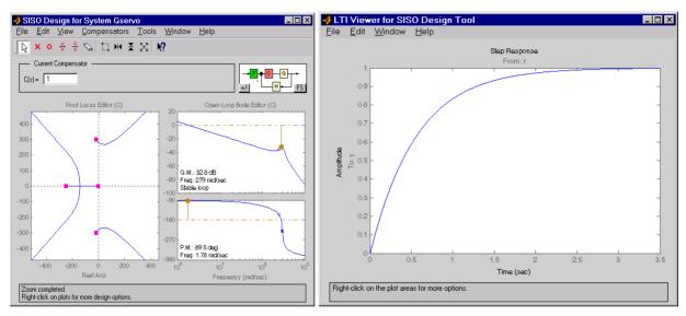
Figure 4-28: SISO Design Tool and Associated LTI Viewer for the Electrohydraulic Servomechanism
