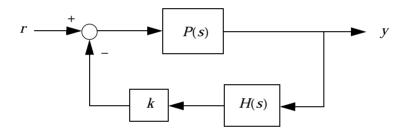
where P(s) is the plant, H(s) is the sensor dynamics, and k is a scalar gain to be adjusted. The closed-loop poles are the roots of
