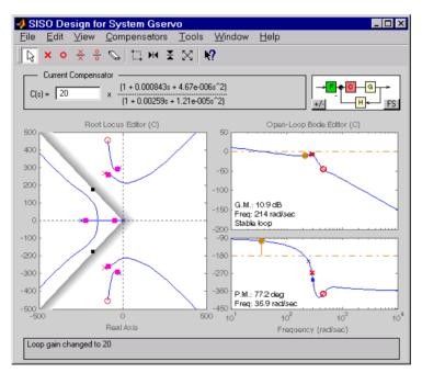
Figure 4-38: Root Locus Displaying 0.707 Damping Ratio Lines
